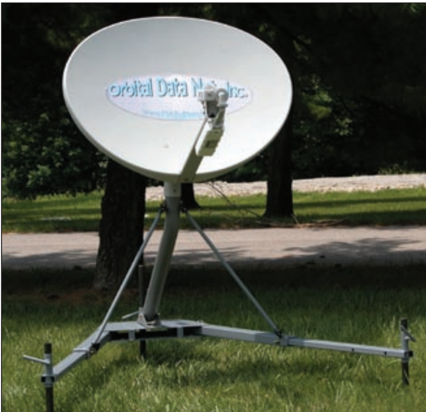
In answering a call from the National Guard, Orbital produces a custom transportable VSAT capable of being transported in the trunk of a car, or the cargo area of a helicopter. This unit can restore communications to a site hit by a national disaster or terrorist activity within minutes.
