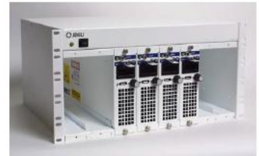
Local Module Chassis Up to 8 Laser Modules
