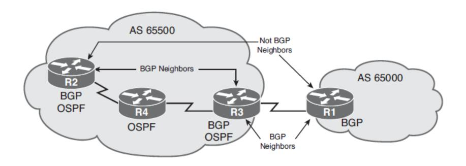
BGP peers can be either internal (iBGP) or external (eBGP) to the autonomous system.
